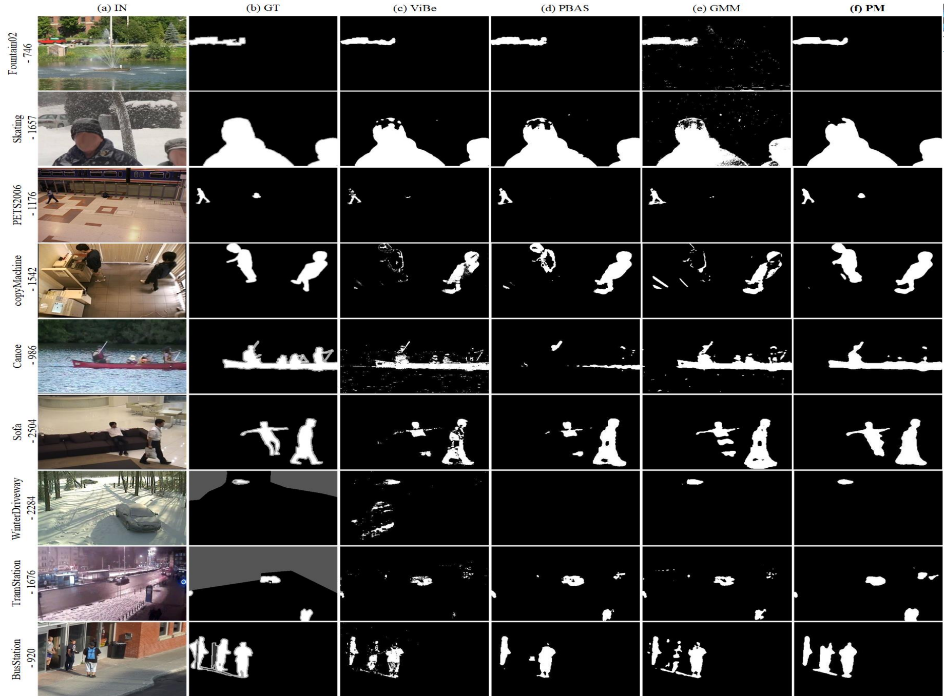
Fig. 8. Foreground detection results of the proposed method and other state-of-the-art methods
